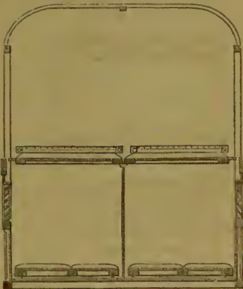
Fig. 9. The Body of the "Rucker" Ambulance—Arranged for four recumbent patients. Assistant-Surgeon U. S. A., has given much study to the subject, and has recently succeeded in introducing not only his ambulance into London, but has also laid the foundations for an ambulance service in that city, where so many thousands are annually injured. His wagon
